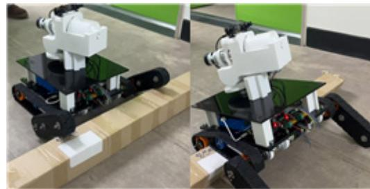
Fig. 1 Vertical Obstacle Traversal Process
