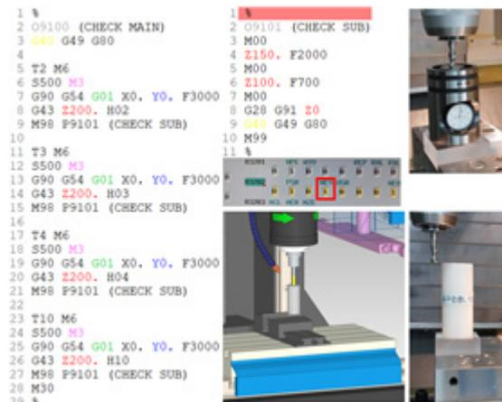
Fig. 3 Setting verification for real machining
