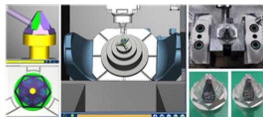
Fig. 4 Simulation, 5-axis machining and results
