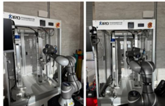
Fig. 1 Robot grasp testing machine
