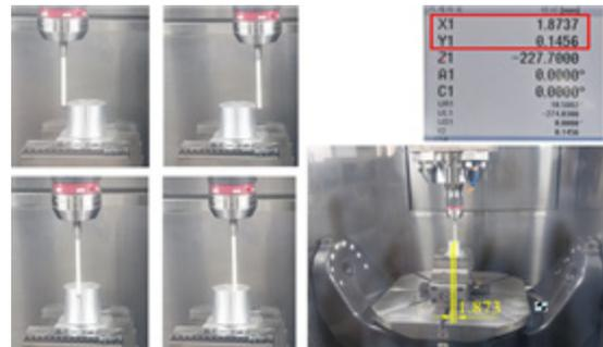
Fig. 2 Eccentricity between table and workpiece center
