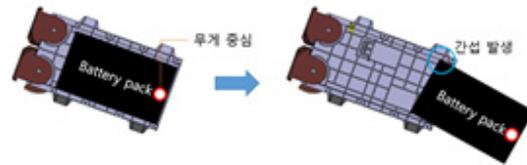
Fig. 2 Rear center of gravity battery ejection separation motion simulation
